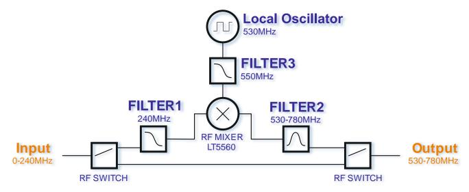
The high performance double balanced active Mixer LT5560 is at the core of the design. This component offers excellent response for low level signals.
